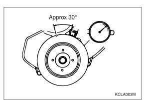
10. Rotate the crankshaft to the right to place the pulley notch to  $5^{\circ}$ .
