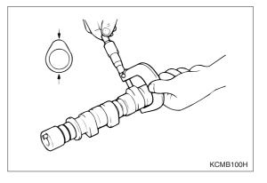
3. Check the cam surface for abnormal wear or damage and replace it if required.
