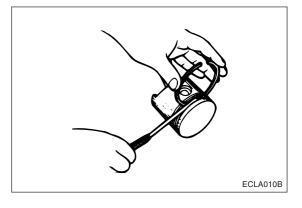
3. Measure the clearance between piston ring and ring home.
