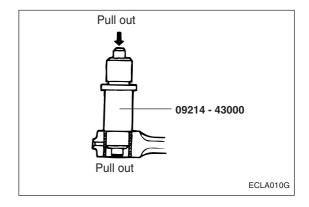
Press-fit the bushing using the special tool.
