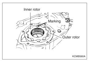
When air pressure of 0.5kg/cm<sup>2</sup> is applied to the oil hole, if there is no continuity, it is normal.
