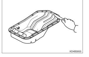
2. Cut the nozzle attached to the liquefied gasket as shown in the illustration. The liquefied gasket comes out with 4mm diameter.
