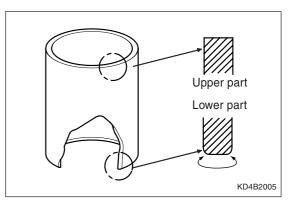
To prevent the cylinder sleeve and cylinder block top surfaces from roughness and bump, cut the cylinder block top surface.
