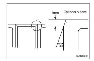
Cylinder sleeve I.D. is processed with 90.08~90.10mm, after press-fitting the sleeve, hone the bore to be within the standard value.
