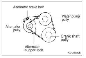
4. When using a tension gauge, move the alternator to the standard tension value.
