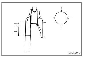
Measure the connecting rod bearing I.D. and crankshaft pin O.D. If the clearance (oil clearance) exceeds the limit, replace the bearing and, if necessary, the crankshaft. Or, grind the crankshaft to an undersize and, at the same time, replace the bearing with an undersize.
