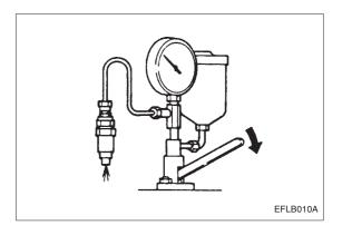
5. If the injection start pressure can not be adjusted by changing the shim thickness, replace nozzle assembly.
