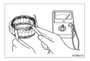
2. Check the coil grounding. Make sure that there is no continuity between the coil and core. Replace the stator assembly if there is continuity.
