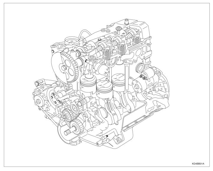
Crankshaft is made of forged steel and supported with main bearing. Pulley attached with torsional damper is installed in the front of crankshaft and flywheel in the rear of it. Silent shaft is installed to both ends of the cylinder block, operated with cog belt and rotated at a double speed of crankshaft.
