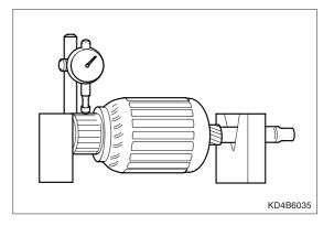
2. Check the outer diameter of the commutator.
