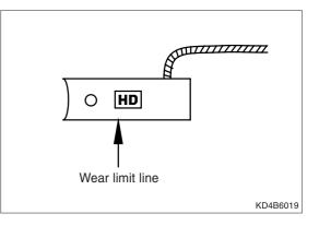
2. Unsolder the brush lead wires, and the brush and spring will come out.
