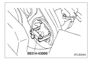
4. Leave the sprocket in the timing belt lower cover with the timing belt engaged.
