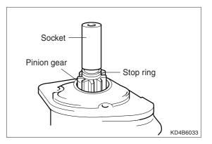
2. Remove the snap ring with a screwdriver, then, remove the stop ring.
