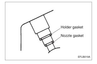
2. Fit a new nozzle gasket and holder gasket into the nozzle holder hole in the cylinder head.
