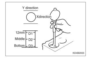
Be sure when boring the cylinder, all sleeves should be removed from all cylinders not to make mistakes during rounding.
