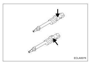
Using Bearing Installer Stopper and Silent Shaft Bearing Puller (09212 - 43300, 09212 - 43100), remove two rear bearings from the cylinder block.
