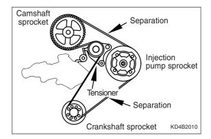
3. Check if all timing marks are aligned correctly.
