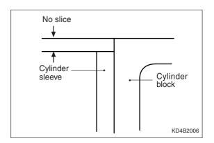
5) Chamfer the cylinder sleeve top end as shown in the illustration.
