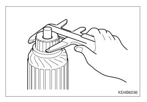
3. Check the depth of the undercut between segments.
