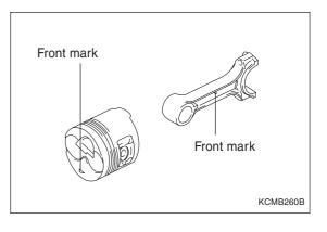
2. Install the snap ring in the following direction.
