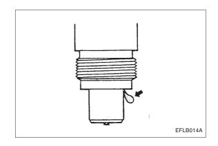
2. If there is leakage, disassemble injection nozzle and replace nozzle tip or entire assembly.
