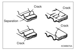
Side of belt cracked Normal belt should have precisely cut side as if produced by a sharp knife.
