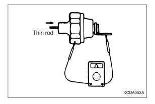
Apply a 0.5 kg/cm<sup>2</sup> pressure to the oil hole. The switch is normal if there is no continuity. Also check for air leaks. If any air leaks are detected, the cause may be a broken diaphragm. Replace the switch if it leaks.
