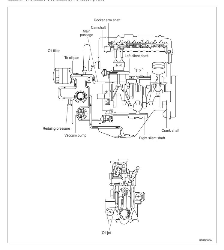
Oil filter is a combined type and full flow filter and bypass filter are built in it. The bypass filter in the full flow filter uses a thick multi-fiber media to filter dirt (soot).
