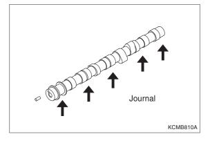
2. Measure the camshaft diameter and bearing inner diameter and if the oil clearance exceeds the limit value, replace the camshaft, cylinder head or both.
