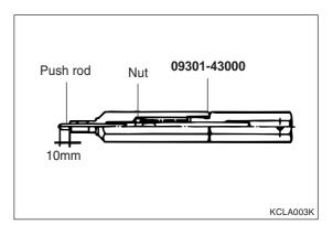
6. Install the dial gauge by installing the special tool to the injection pump.
