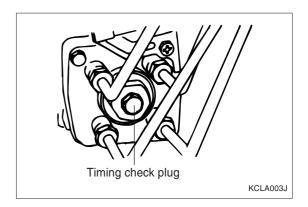
5. Before installing the special tool, check that the push rod is jutted out about 10mm. Protrusion of the push rod is adjusted by the inner nut.
