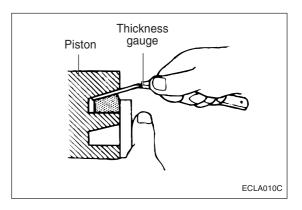
4. Place a piston ring in the cylinder bore and set it square by pushing it down with piston.
